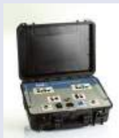
20A DC BOOSTER FOR WINDING RESISTANCE TEST
